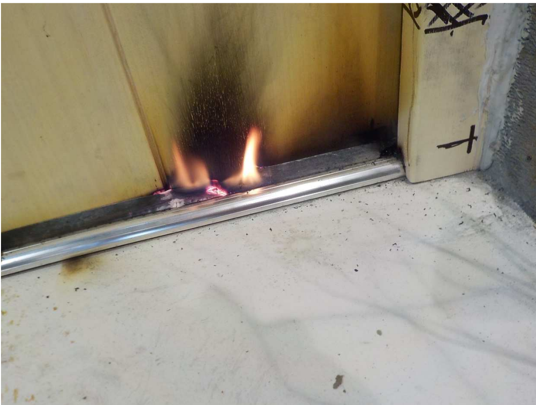
Photo 2.2.8 – left-hand doorset after 35 minutes
