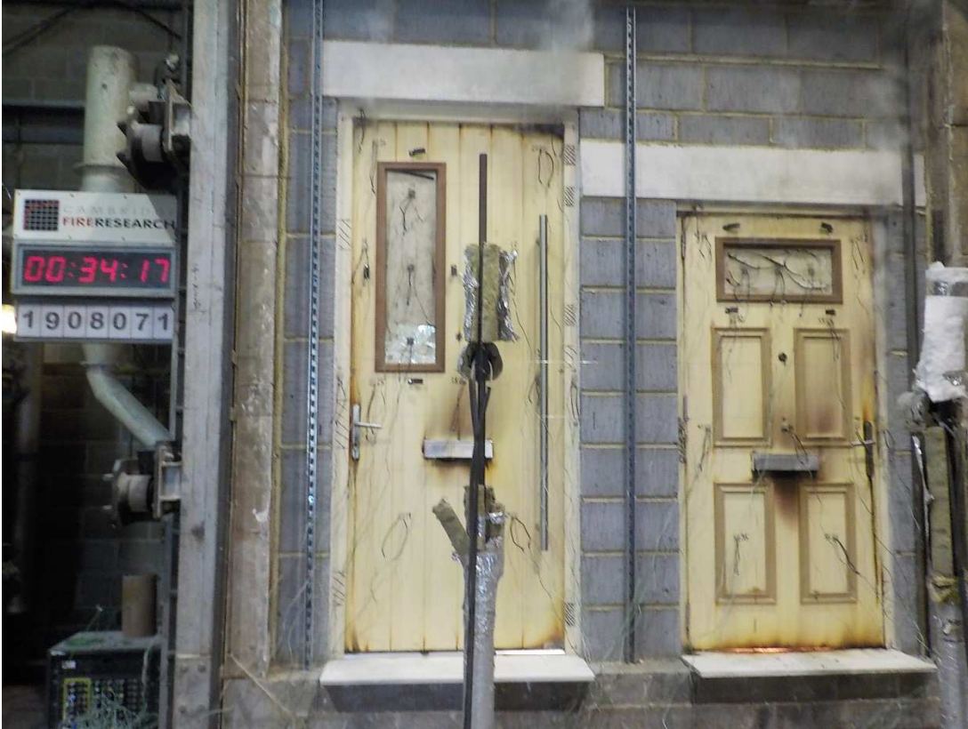
Photo 2.2.8 – left-hand doorset after 35 minutes
